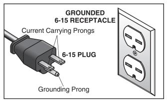
Figure 5. Typical 6-15 plug and receptacle.
